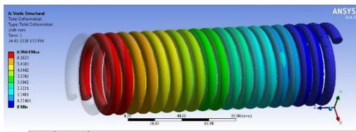
Fig 12 Total Deformation
