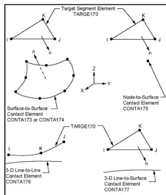
Fig 3 TARGE170 Geometry
