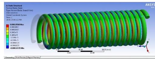
Fig 7 Normal Elastic Strain
