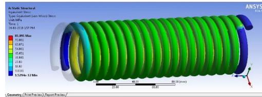
Fig 14 Equivalent Stress (von Mises)
