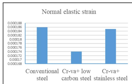
**Fig 31 Comparison of Normal Elastic Strain**
