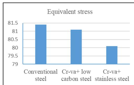
**Fig 30 Comparison of Equivalent Stress**
