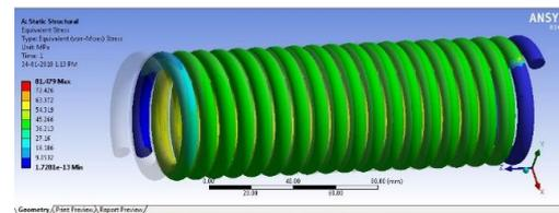
Fig 6 Equivalent Stress (von Mises)
