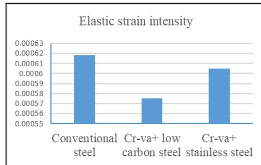
**Fig 29 Comparison of Elastic Strain Intensity**
