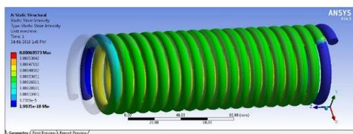
Fig 21 Elastic Strain Intensity
