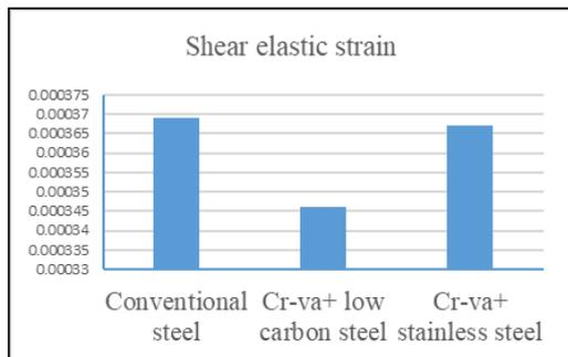
**Fig 33** Comparison of Shear Elastic Strain
