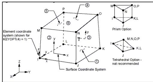
Fig 2 SOLID45 Geometry
