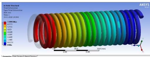
Fig 20 Total Deformation
