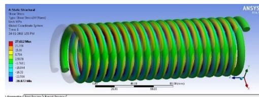
Fig 18 Shear Stress
