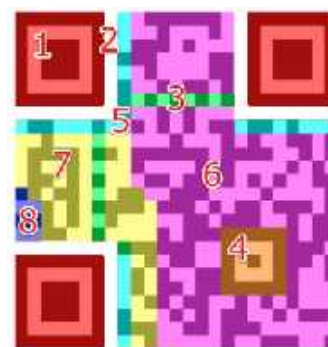
Figure 2. Parts of a QR Code
