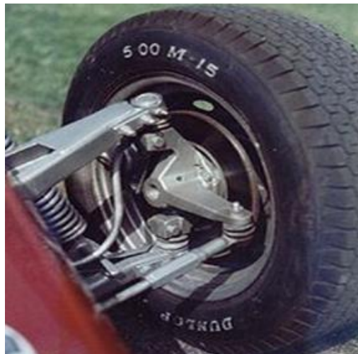
Part of steering mechanism: tie rod, steering arm, king pin.
