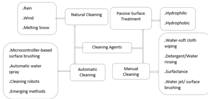
Fig 2 Different cleaning methods for removing dust from solar collectors [15]
