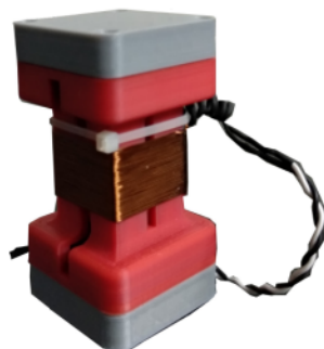
Figure 3 Magnetic Levitation Energy Harvester (final design)
