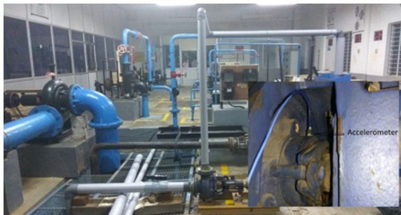
Figure 2: Position of Accelerometer
