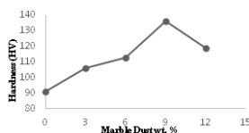
Figure 7 Variation of Hardness with wt.% of MD
