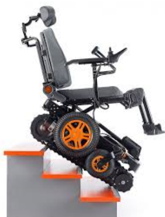
Fig.1. (Topchair-S escalator model stair climber)
