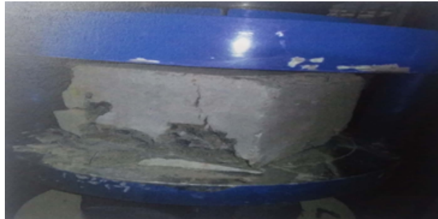
Fig2.Compressive strength test for cube
