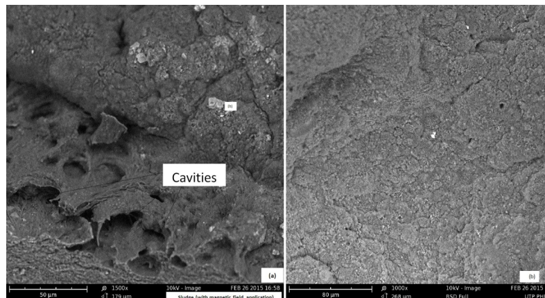
Figure 4 SEM microstructure of the granule. Cavities that present between bacteria are clumped inside the granules which been exposed with magnetic field (a) sludge after granule development; scale bar = 50 m (b) raw sludge; scale bar = 80 m
