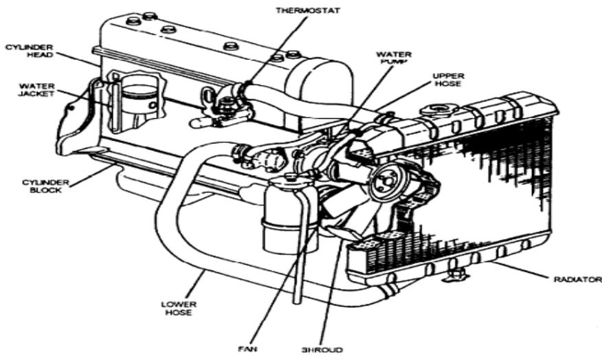
Figure 3.1 Components of cooling system
