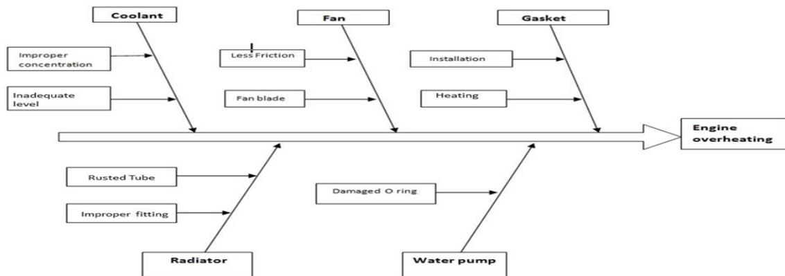
Figure 5.1 cause & effect diagram
