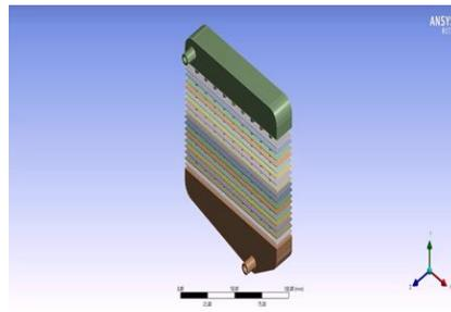
Figure 6.1 model of the radiator
