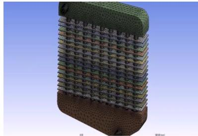
Figure 6.2 mesh model of radiator
