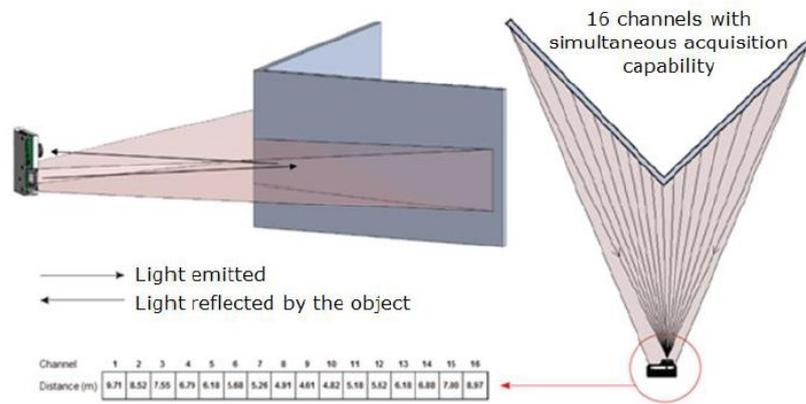
Fig. 1. Representation of Liddar sensor working
