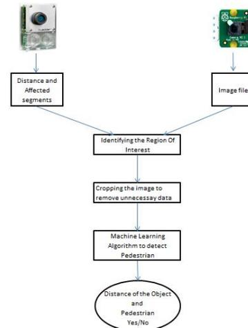
Fig. 5. Data fusion process flow representation
