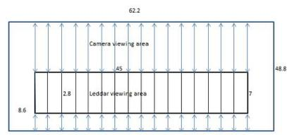
Fig. 4. Representation of Projection of Liddar Data over Camera Image
