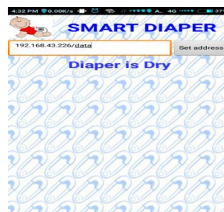
Figure 6 displays the status of the diaper as dry when the diaper is not wet by the liquid.
