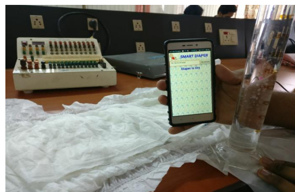
Figure 5 Final Output When sensing is being completed by three sensors alert message will be delivered to the corresponding device.
