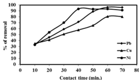
Fig 3 : Effect of contact time onto Pb(II), Cu(II) and Ni(II) metal ion by Cell- TA (Optimized adsorbent dose = 40 mg/L, optimized pH=6 and Optimized initial metal ion concentration = 100 mg/L)
