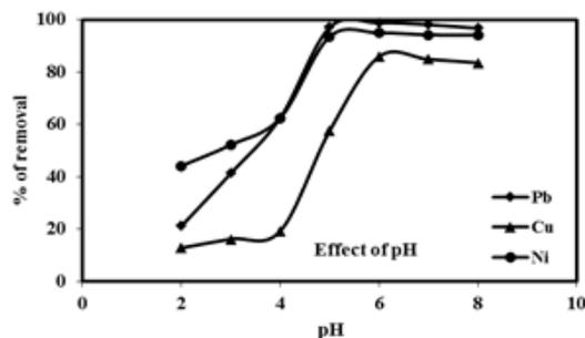
Fig 2: Effect of pH onto Pb (II), Cu (II) and Ni (II) metal sorption by Cell-TA (Initial metal ion
