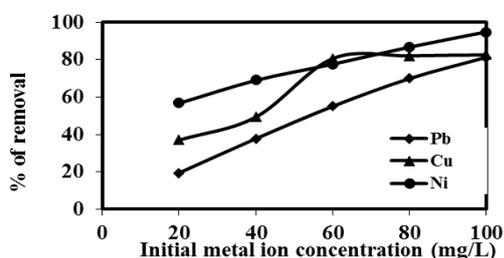
**Fig 4 : Effect of initial metal ion concentration onto metal sorption Pb(II), Cu(II) and Ni(II) on to Cell-TA (Optimized adsorbent dose = 40 mg/L, optimized pH=6 and Contact time=60 min)**
