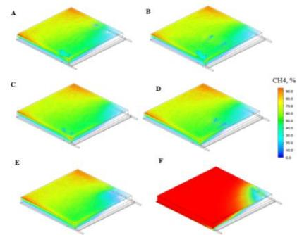
**Figure 2. Methane concentration (%) with various arrangements of degassing wells**
