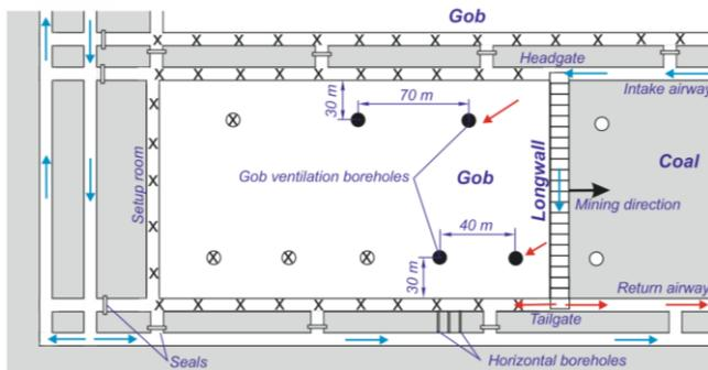
**Figure 1. Scheme of ventilation and arrangement of degassing wells**
