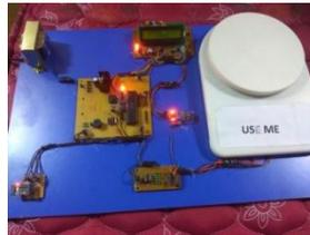
Fig 3: The IOT based garbage monitor system setup
