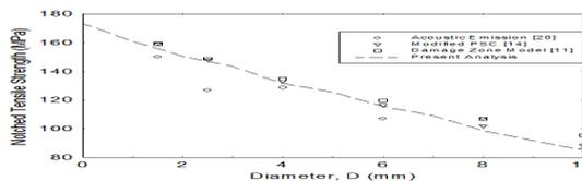
Figure.7 Comparison of fracture models on the notched tensile strength estimates of 225x25.2x3mm C/C composites.
