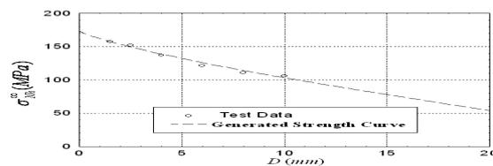
Figure.5 Variation of notched strength ( $\sigma_{Nh}^\infty$ ) with hole-diameter.
