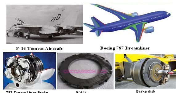
**Figure 1.** Components of C/C composites used in aircrafts [2, 3]
