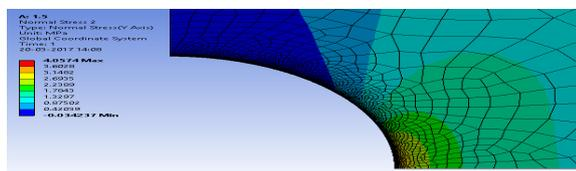
**Figure.2** Stress contour near the central opening of the infinite width C/C composite laminate under a tensile stress of 1 MPa.
