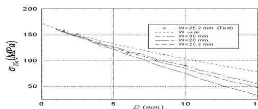
Figure.6 Notched strength ( $\sigma_{Nh}$ ) variation with hole-diameter for different plate width.
