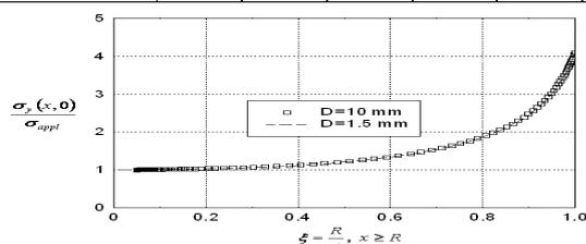
**Figure.3** The normal stress distribution  $\sigma_y(x,0)$  adjacent to the central opening in an infinite width C/C laminate under a uniform stress  $\sigma_{appl}$ .
